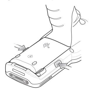
2. Remove the battery from the battery compartment.
