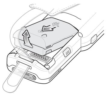
3. Align the battery into the battery compartment.
