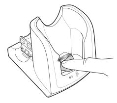
2. Peel and remove the adhesive from the back of the adapter.
