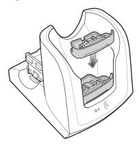
4. Insert the MC33XX or MC3300x mobile computer into the MC32N0 cradle.
