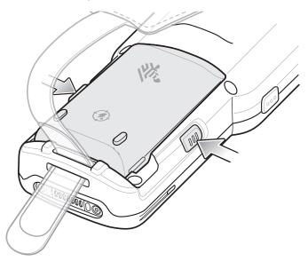
2. Remove the battery from the battery compartment.
