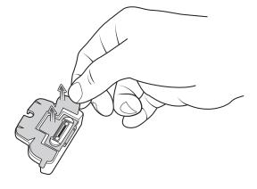
3. Insert the adapter into the MC32N0 cradle and adhere to the bottom of the cradle.
