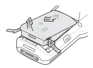
3. Align the battery into the battery compartment.
