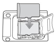
5. Close the microSD card holder and slide the microSD card holder to the Lock position.
