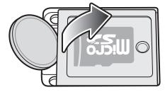
2. Slide the microSD card holder to the Open position.
