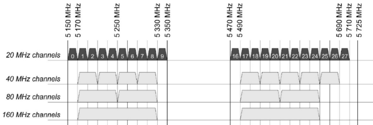
Figure 3: Channel Bonding for option 2
